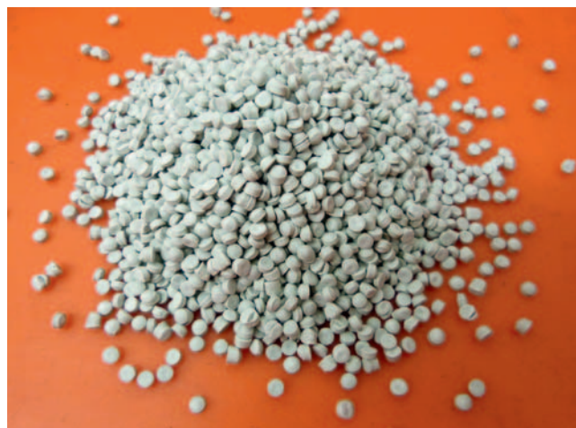
Figure 5. Washed shreds of severely contaminated agricultural film (left) processed with Corema 1108 T (filter system Erema SW 4/134 RTF, 300 µm) to make recycled pellets with 75 % CaCO 3 content
