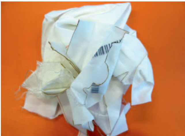
Fig. 7. PA6.6 fabric/production waste from airbag production
